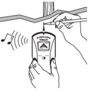
Without releasing Power button, continue scanning beyond marked spot until some segments of the arrow turn off. Slide unit in reverse direction to locate other edge of stud.
