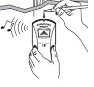
**⚠ WARNING** Electrical field locators may not detect live AC wires if moisture is present in the wall, or if wires are more than 50 mm from the scanned surface, in plastic conduit or behind a plywood shear wall or metallic wall covering.
